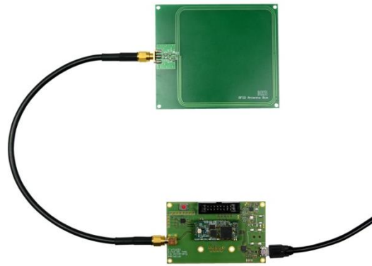
Exemplary arrangement: Evaluation kit with RFID OEM module and 5cm PCB RFID antenna
